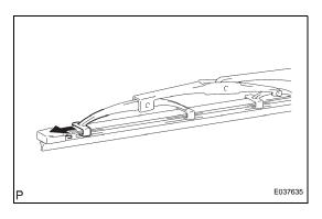
(b) Install the wiper rubber with its head portion (swelled portion) facing the arm bearing.
