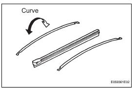
(b) Remove the 2 wiper rubber backing plates from the wiper rubber.
